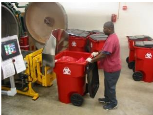
Operator rolls cart to Autoloader
